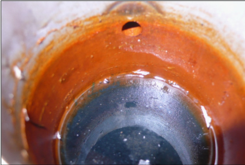
Figure 7. Venting hole in the 7" tube.
