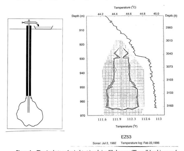
Figure 1. - The simplest mechanical test in a brine-filled cavern (The well head is opened to atmosphere and the brine flow expelled from the cavern is thoroughly measured).
