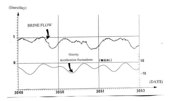
Figure 4.- The brine flow fluctuations have been corrected from ground level temperature and atmospheric pressure variations. (The periodic character of the corrected fluctuations appear clearly.)
