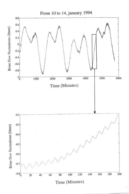
Figure 6.- Brine flow fluctuations observed during four days.
