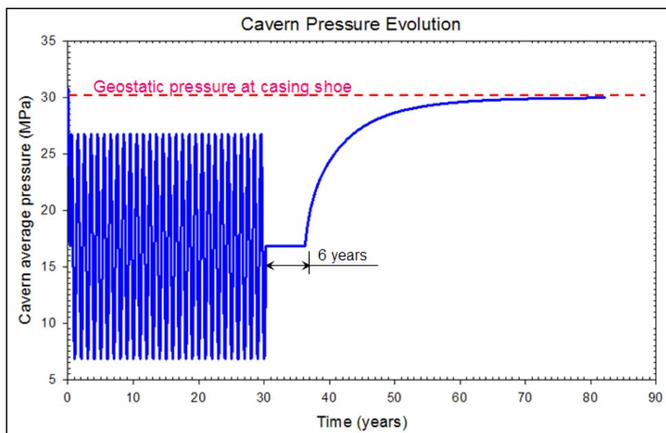
Figure 11 – Cavern pressure evolution, Case 6 — 6-year waiting period, no gas,  $K_{salt}^{perm} = 10^{-21} \text{ m}^2$ .
