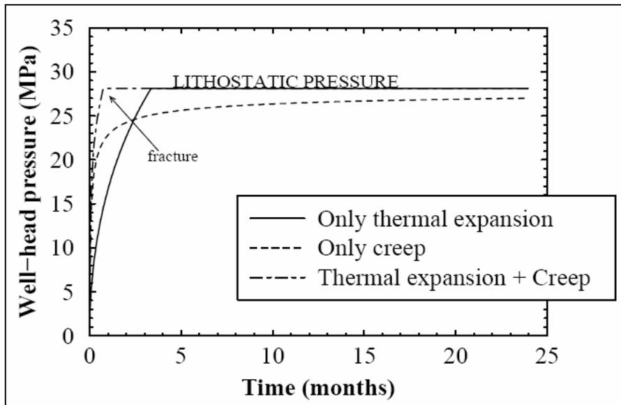
Figure 1 - Computed pressure evolution in a closed cavern. Brine thermal expansion leads to fracture.
