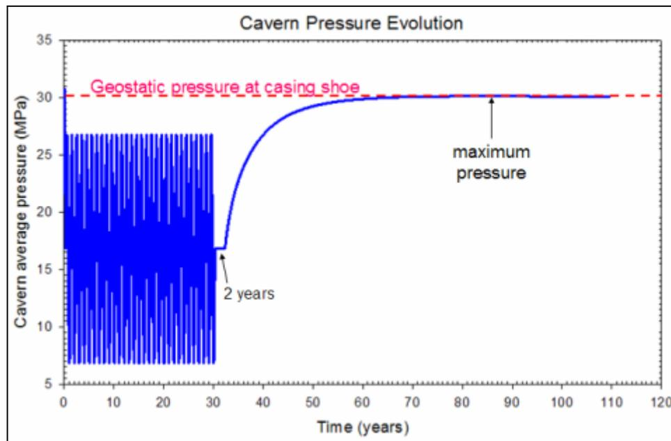
Figure 12 – Cavern pressure evolution, Case 6 — 2-year waiting period,  $V_g = 900 \text{ m}^3$ ,  $K_{salt}^{perm} = 10^{-21} \text{ m}^2$ .
