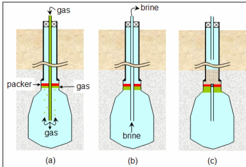
**Figure 2 - Increasing cavern compressibility: (a) gas is injected below the packer; (b) brine is withdrawn to release pressure build-up; (c) the central tubing is sealed and cement is poured into the well.**
