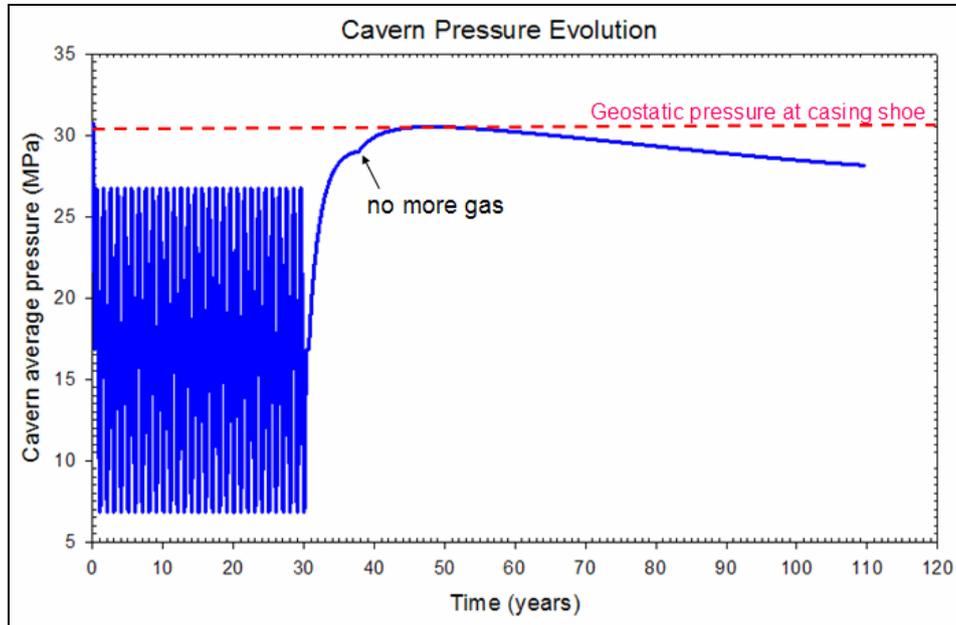
Figure 10 – Cavern pressure evolution, Case 5 — 6-month waiting period,  $V_g = 300 \text{ m}^3$ , small leak.
