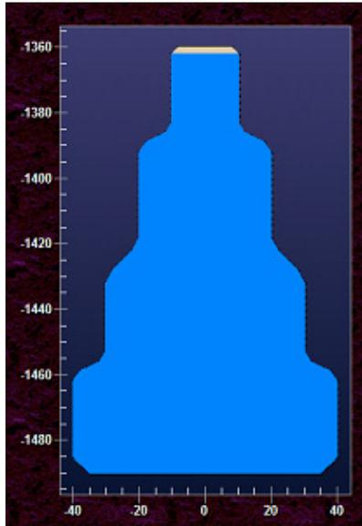
Figure 3 - Cavern shape – Nitrogen cap volume is  $V_g = 300 \text{ m}^3$  in this example.
